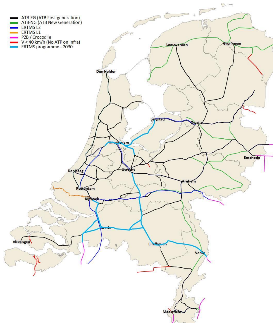
Figure 2. Railway lines in the Netherlands with ATP systems. Light blue: ERTMS in the 2030 scope
